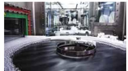
IPS is providing CQV services on the Bavarian Nordic Sterilization Tunnel Exit Turntable to Enter Filling Line
